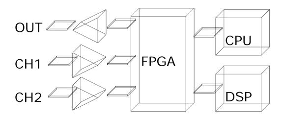
This general purpose structure provides a versatile hardware platform that can be configured by firmware to provide a variety of test functions, including:
