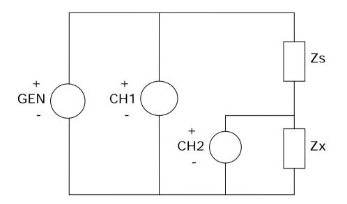
For "divider Zx low" connection, shown above, the total voltage is measured by CH1 and the voltage arising from the potential divider effect of Zs and Zx is measured by CH2. Notice that all the negative terminals are connected together.
