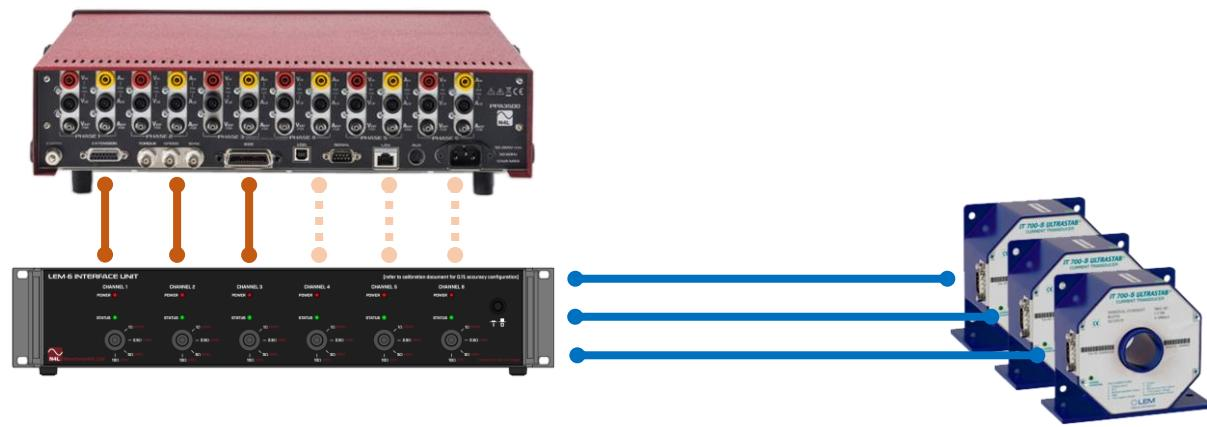
Where multiple burden resistors are not required, the CT current is above 707 Arms or the distance between the power analyzers and CT's is above 6m, the LEM-1 Interface powered by one of our LEM-1 Power Modules provides the solution.
